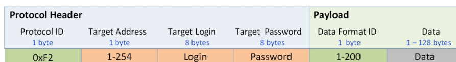
Figure 9 - Protocol for exchanging data on the same network without routing. ID: 0xF2
