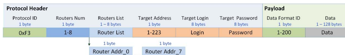
Figure 10 - Protocol for exchanging data on the same network with routing. ID: 0xF3
